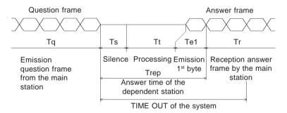
The time beyond which the device does not answer is called "TIME OUT". It depends on the transmission parameters (speed, format) and the type of the function asked (reading, writing). This time must be defined by the user and must be superior to the answer time of the device.
